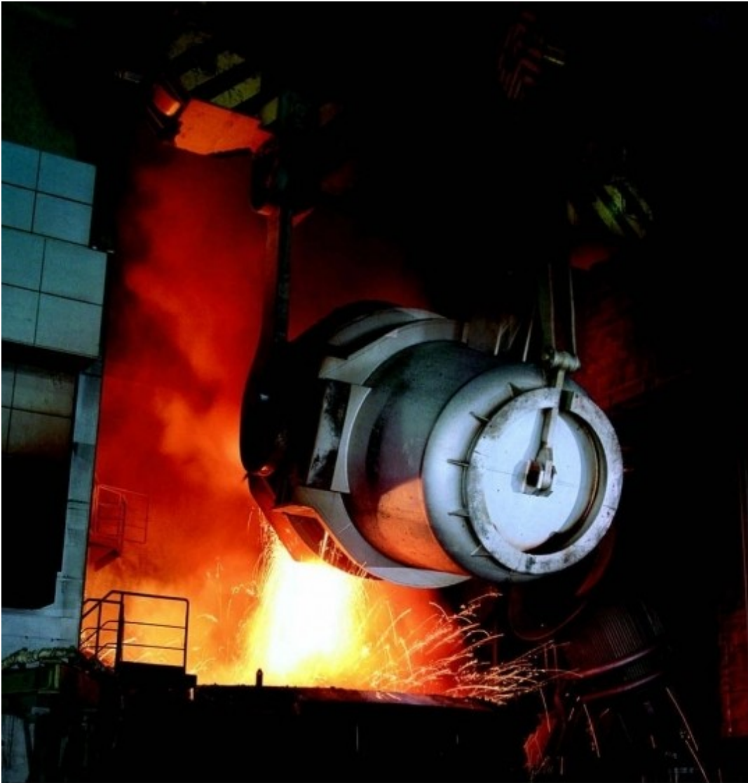
Chargieren von Flüssigstahl in einem Elektroofen im Edelstahlwerk Shanghai Baosteel No. 1 Source: SMS group Charging of liquid steel into an electric arc furnace at the stainless steel meltshop of Shanghai Baosteel No. 1
